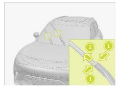
Hold the wiper arm with one hand, press the clip inward along the direction of the arrow 1, and pull the blade out along the direction of the arrow 2 with the other hand.
