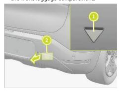
Press the lower point of the triangular indicator inward to remove the tow bar cover 2.
