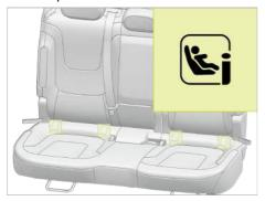
The outboard second row seats are equipped with ISOFIX/i-Size anchor points. Flip away the child restraint system anchor point covers and the anchor points are located on the seat cushions (as the figure shows above).
