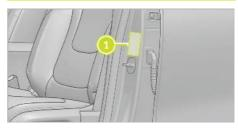
The tyre pressure table is located on the front of left B pillar 1.
