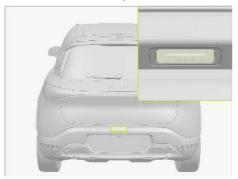
Bring along the keyfob and press the button on the liftgate. **Manual liftgate:** press the button on the liftgate to unlock and pull the liftgate upward slightly, the liftgate opens up automatically and gradually.
