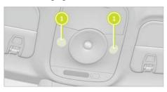
**ON/OFF:** touch or press the reading light depending on the vehicle configuration. Depending on the vehicle configuration, press and hold the physical switch of the reading light to adjust the light brightness.
