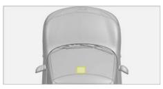
The rain light sensor is located on the upper part of the front windshield, and the automatic wipers/automatic headlamp/automatic climate control controls the corresponding functions through this sensor.
