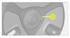
Insert the hook into the wheel trim cover hole and pull it outward to remove the wheel trim cover.
