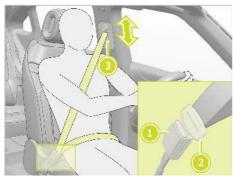
Always insert a seat belt tongue 2 into the buckle 1 of the corresponding seat.
