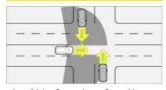
When driving forward out of a parking space or through an intersection with impaired vision, Front Cross Traffic Alert alerts the driver to brake to reduce the risk of forward side impact.
