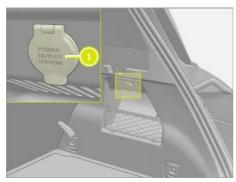
Lift up the cover 1 and insert the device connector.
