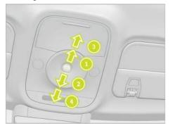
To open the sun shield manually: push the switch in the direction of the arrow to the first resistance point, the sun shield opens manually.
