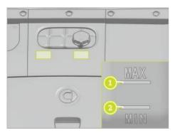
If the coolant level is lower than the marked position 2, inspect or top up coolant at a smart Authorized Service Partner
