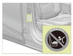
The label is visible on the passenger side B pillar when the front passenger door is opened.
